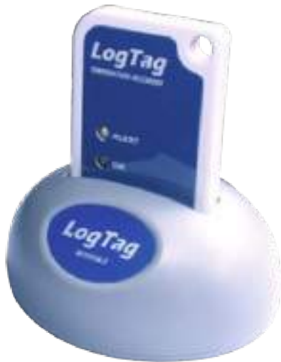
Figure 9: Standard interface cradle with LogTag®
